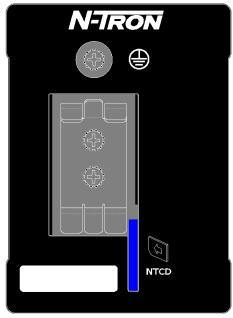
The configuration device is inserted in the back of the 710FX2.
